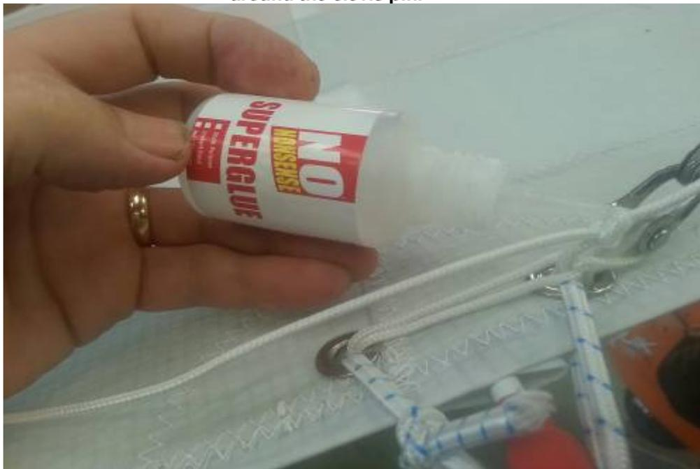
**Fig 5 loop the cord through both eyelets, tie the ends off around the clevis pin with a reef knot. Use pliers to get it really tight. Apply cyanoacrylate to the knot ( superglue). .
